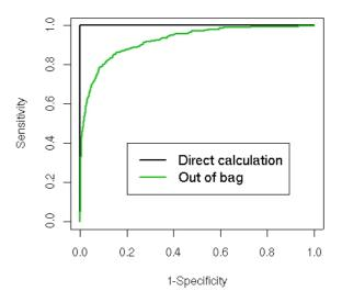
Figure 8. ROC curves for Random Forest for the training set built from the probability estimates directly calculated by the use of the chosen model (black) and from the out-of-bag probability estimates (green).
