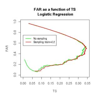
Figure 4. FAR as a function of TS for the test set for logistic regression trained with train (green) or train.sample (red) with 500 discretization points.
